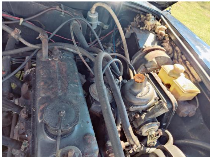
Evidence of rodent residency beneath the bonnet.
