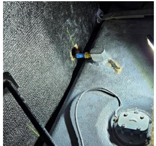
No fuel line from the tank to the pump equals no fuel to the engine (photo by Tim Garrold).
