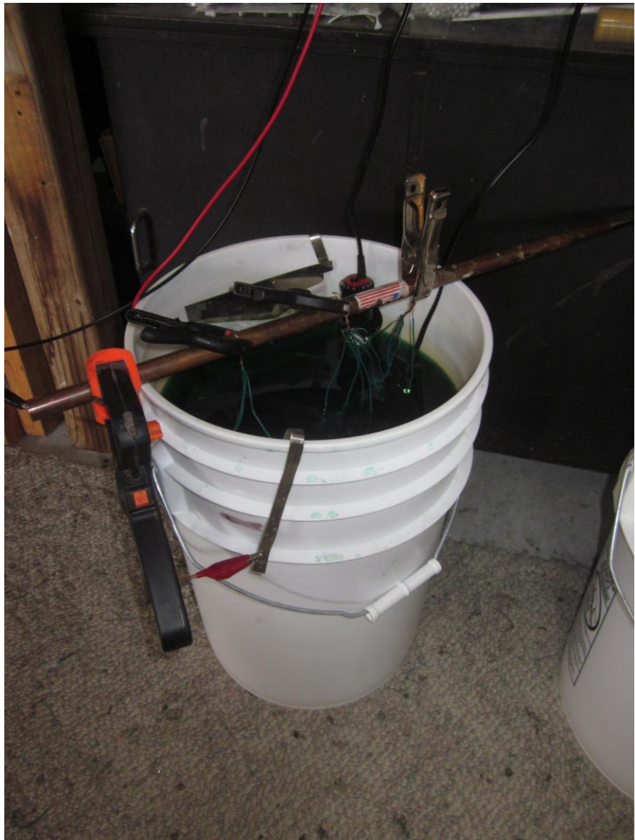
Carburetor parts undergoing nickel plating during one of my first attempts.
